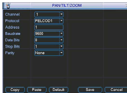
Figure 45 DVR PTZ setup
